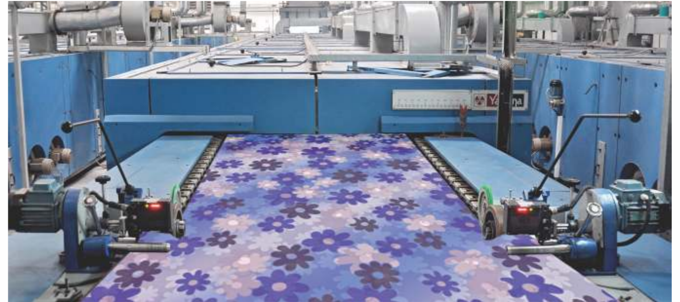
Diversified chain Inlet lengths as 3 m, 4.5 m, 6 m for finishing processes of woven, knitted and home textile fabrics.
